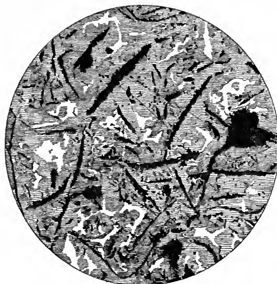
FIG. 27.—Graphite in Grey Cast Iron.
